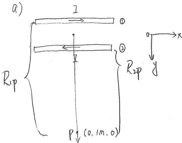
$$\begin{aligned} \vec{B}_p &= \frac{\mu_0 I}{2\pi R_{1p}} \hat{z} - \frac{\mu_0 I}{2\pi R_{2p}} \hat{z} \\ &= \frac{4\pi \cdot 10^{-7} \cdot 2}{2\pi (1\text{m} + \frac{1\text{cm}}{2})} \hat{z} - \frac{4\pi \cdot 10^{-7} \cdot 2}{2\pi (1\text{m} - \frac{1\text{cm}}{2})} \hat{z} \\ &= \frac{4 \times 10^{-7}}{(1+0.005)} \hat{z} - \frac{4 \times 10^{-7}}{(1-0.005)} \hat{z} \end{aligned}$$
