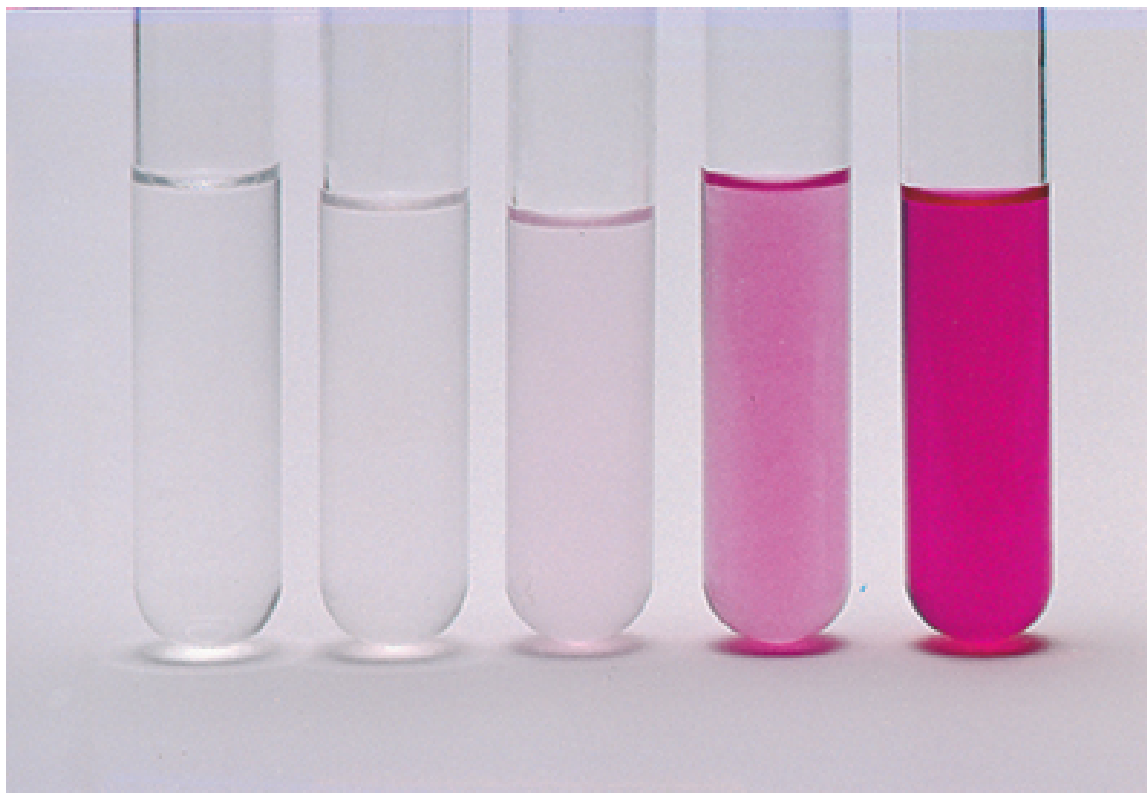
FIGURE 12.10 The stoichiometric point of an acid–base titration may be detected by the color change of an indicator. Here we see the colors of solutions containing a few drops of phenolphthalein at (from left to right) pH of 7.0, 8.5, 9.4 (its end point), 9.8, and 12.0. At the end point, the concentrations of the conjugate acid and base forms of the indicator are equal.
