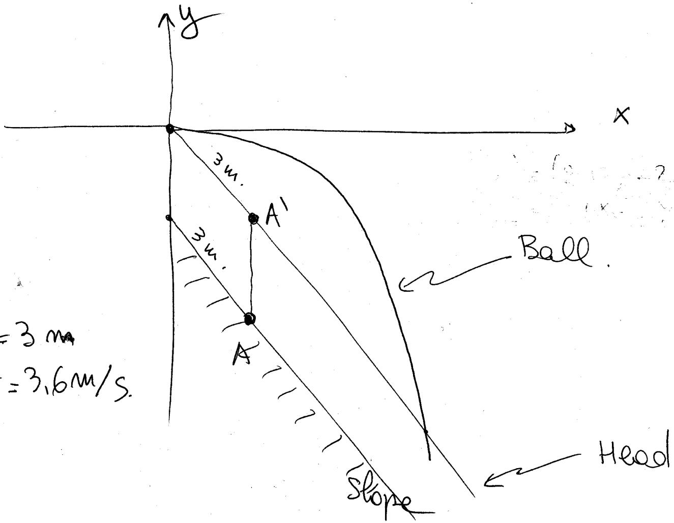
$$\text{Ball: } x_1(t) = v_0 t \quad y_1(t) = -\frac{1}{2} g t^2.$$
