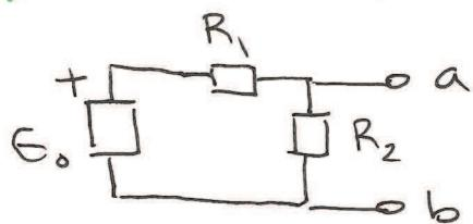
$$U_{E_o} = \frac{R_2}{R_1 + R_2} E_o \quad (\text{spänningssplitning})$$
