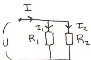
$$\left. \begin{array}{l} I_1 = \frac{U}{R_1} \\ I_2 = \frac{U}{R_2} \end{array} \right\} \text{Ohms lag}$$
