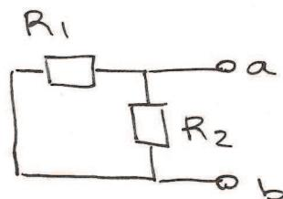
$$R_E = \frac{R_1 R_2}{R_1 + R_2}$$
