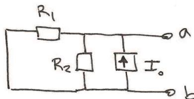
$$U_{I_o} = \frac{R_1 R_2}{R_1 + R_2} I_o$$
