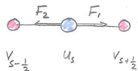
$$F_1 = C(v_{s+\frac{1}{2}} - u_s), \quad F_2 = C(u_s - v_{s-\frac{1}{2}})$$
