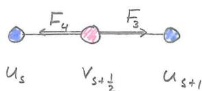
$$F_3 = C(u_{s+1} - v_{s+\frac{1}{2}}), \quad F_4 = C(v_{s+\frac{1}{2}} - u_s)$$
